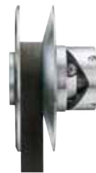
Variable-speed drives with asymmetrical variable speed pulleys, „Becker” system
